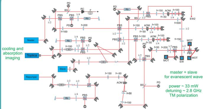
IO - optical isolator, Rb - rubidium cell, PBS - polarization beam splitter, f - lens, PD - photodiode, BS - beam splitter, AOM - acousto-optic modulator, F - fiber,  $\lambda/2$ ,  $\lambda/4$  - half- and quarter-wave plate
