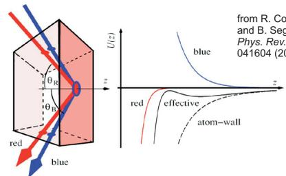
effective attractive potential created by two laser beams (red-detuned and weaker blue-detuned from atomic transition) [3]:
