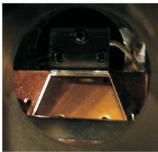
prism in the vacuum chamber - side view
