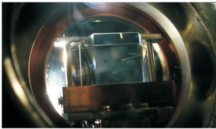
prism in the vacuum chamber - top view
