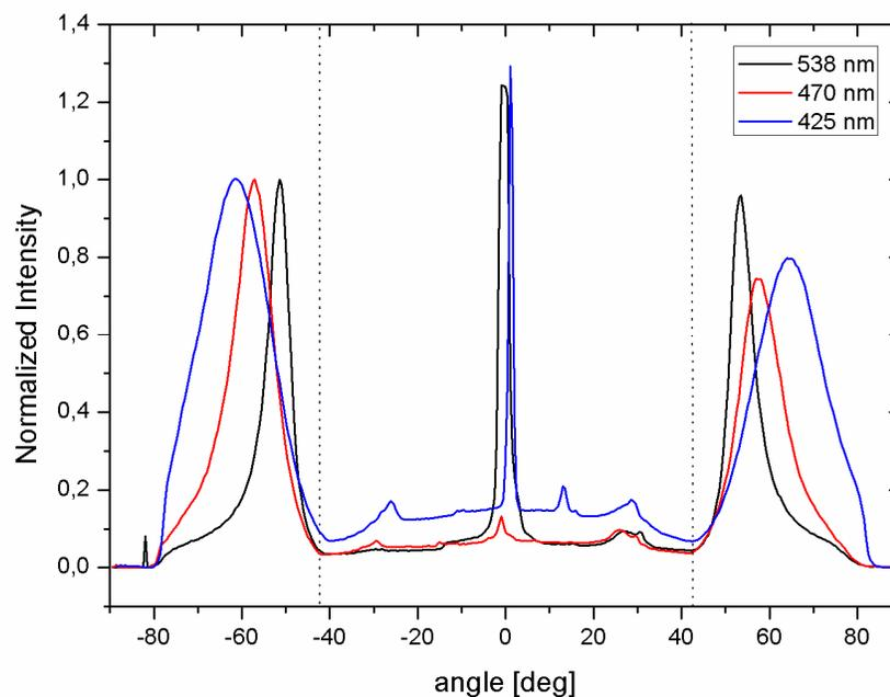
Figure 2. Leakage radiation as a function of  $\Theta$ . Excitation wavelength was 325 nm, and detection was at 425, 470 and 538 nm, respectively. Vertical dotted lines indicate positions of the critical angle.
