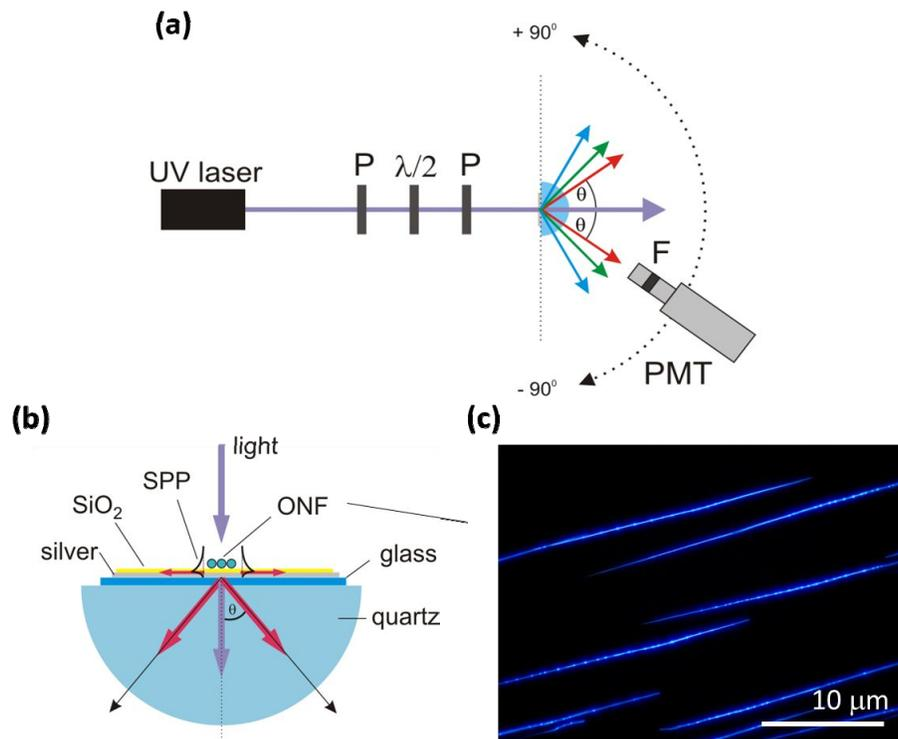
Figure 1. (a) Experimental setup; P - polarizer,  $\lambda/2$  - half-wave plate, F - filter, PMT - photomultiplier. (b) Zoom on the half-sphere with the sample mounted on the flat side; ONF - organic nanofiber. (c) Epifluorescence microscopy image of *p*-6P nanofibers upon UV excitation.
