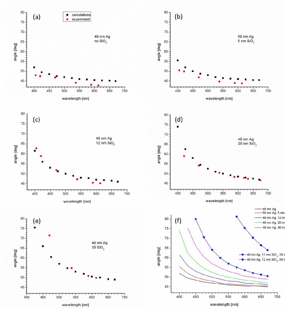
Figure 3. Angular dispersion curves, both calculated and measured for various layer configurations. (a) to (e) are measurements (red dots) and calculations (black squares) for various thicknesses of SiO<sub>2</sub>. (f) summarizes the calculations (solid lines) and includes also calculations using two different p6P thicknesses (lines with symbols).
